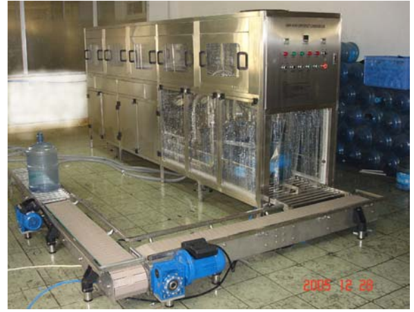
Right: WFC300 with the optional conveyor and roller system allowing the machine to be run by one operator.
